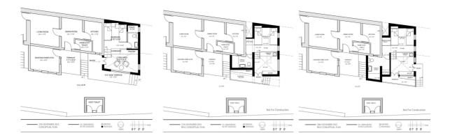
At this stage, it was decided to extend the footprint of the home-stay one foot further, (totalling 15feet or 4500mm from the wall of the hosts' kitchen) in order to create a more spacious layout- in particular, a wider terrace was desired. This led to the creation of Rev4, what we consider the most evolved- where the bathroom is rotated back to its position in Rev2 and a generous volume is allowed for study/lounge/pantry.
